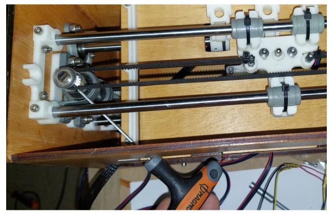
• Loosen the pulley on the vertical axis to release the upper carriage.
