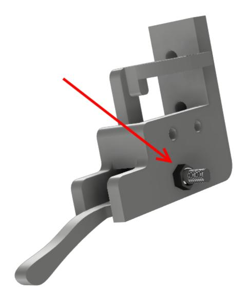
• Assemble the limit switch and the SWITCH\_Y\_support using M2.5-14 screws and M2.5 NYL nuts.
