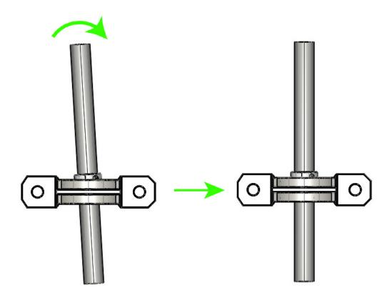
• Screw the KP08\_support and the KP08 on the body a bit with the M5-25 screws, M5 washers and M5 NYL nuts.
