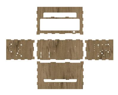
• Glue the notches, assemble the 5 parts and hold them in place with painter's tape the drying time recommended by the manufacturer.
