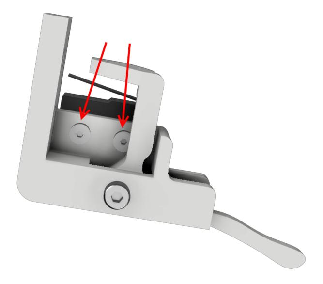
• Position the M3-12 adjustment screw on the lever ENDSTOP\_Y\_LEVER
