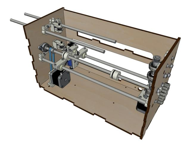
• Thread the top trolley over the rods.
