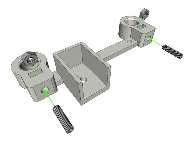
• The end of the screw must not protrude in the passage of  $\emptyset$  8mm bars.
