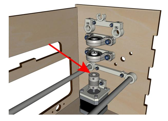
• Thread the 100mm linear shaft from the top through the KP08 and into the coupler.
