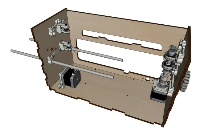
• Thread the switch and its support on the  $\emptyset$ 8mm bar on the back side.
