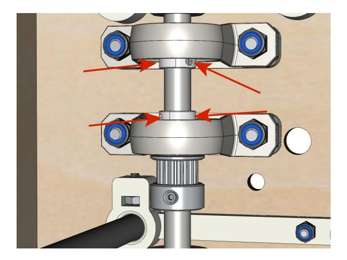
• Make sure that the axle rotates easily and that the motor does not oscillate. If necessary, loosen the motor and support screws on the body to give them play and re-align.
