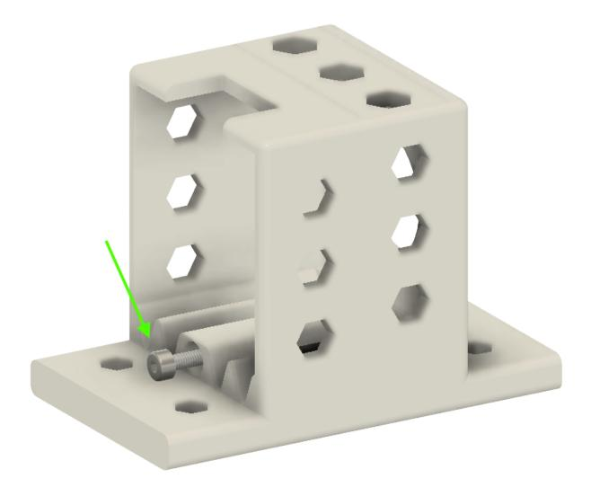
• Fix the part **YMOTOR\_support2\_200** on the previous set with a M3-12 screws.
