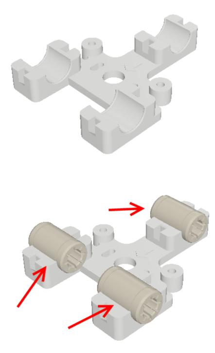
• attach the IGUS bearings with fixing collars
