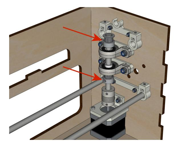
• Screw the 2 screws at the top of the coupler onto the vertical axis.
