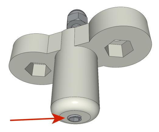
• Assemble the FEMALE\_shape on the TOP\_trolley with the M3-12 screws, the M3 washers and the NYL M3 nuts.
