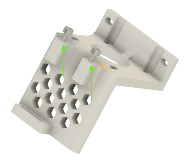
• Fix the motor in its support with 4 M3-8 screws. Do not tighten the screws, the motor must be free to move, it will be tighten later.
