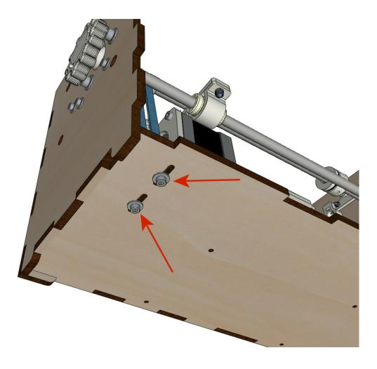
• Tighten the 2 screws of the pulley of the axle.
