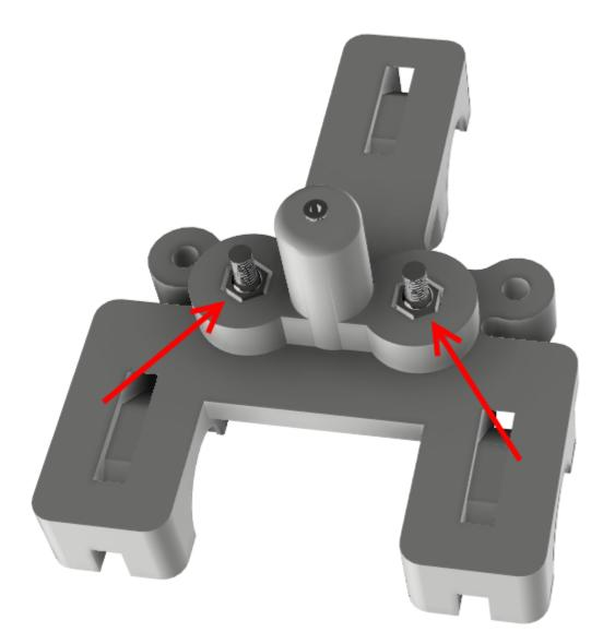
• Position the IGUS bearings on the TOP\_trolley part.
