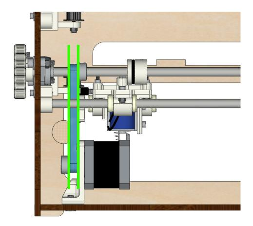
• Move the Y motor / support assembly along the oblong holes under the body to tension the closed belt and tighten the 2 screws.
