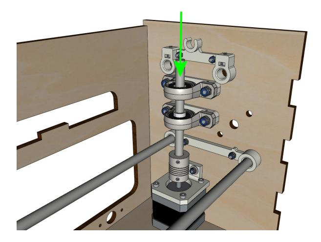
• Rotate the linear shaft by hand to ensure that all elements are aligned and that the spindle continues to rotate freely.
