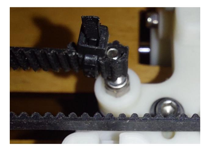
• Pass the belt in the free pulley then the pulley of the vertical axis.
