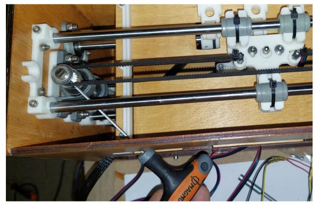
• Loosen the pulley of the upper carriage on the vertical axis to free the top carriage.
