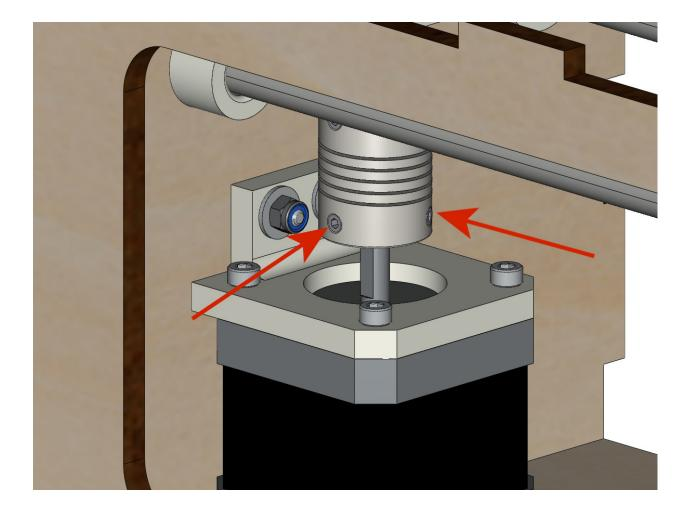
• Thread the 100mm axle into the KP08, the pulleys (respecting their positions) and the coupler.
