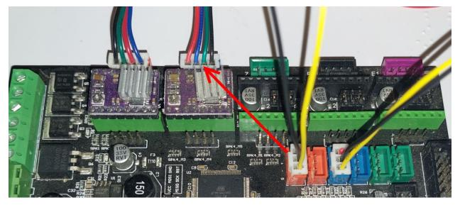
• The Y motor (paper) must be plugged into the right connector (blue)
