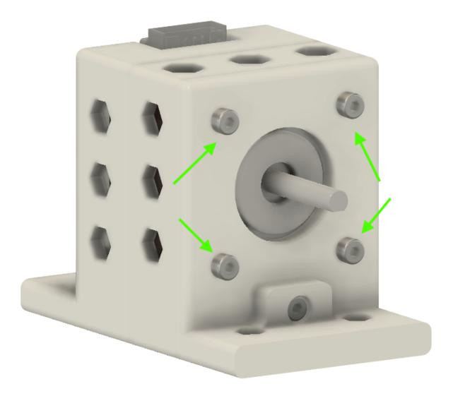
• Insert the 4 NYL M3 nuts into the engine mount. Hold them in place with a small piece of painter's tape.
