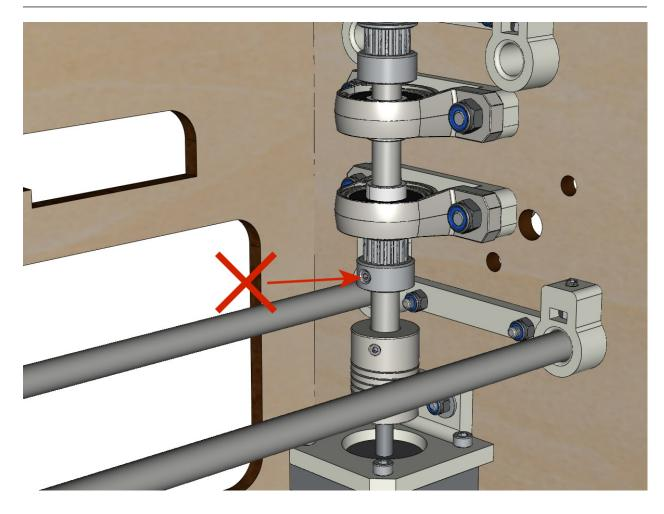
**Note:** For now, do not tighten the pulley bolts on the axle.
