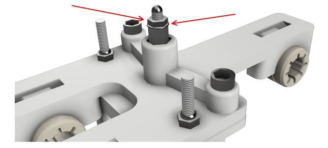
• Fit a washer and tighten the M3 lock nut, ensuring that the stylus screw does not move into the spacer at the same time. The washer prevents the jam nut from getting caught in the spacer guide.
